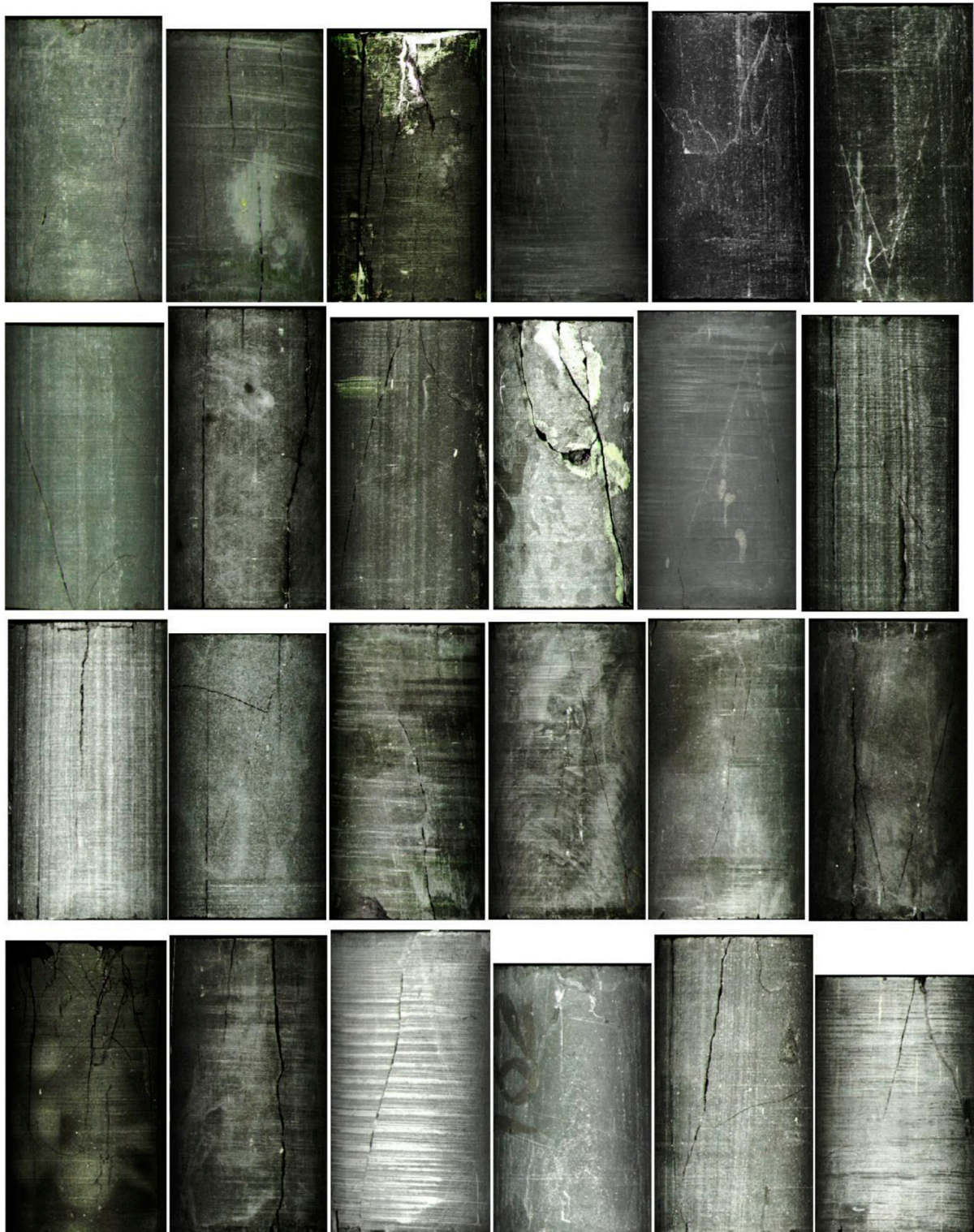
FIGURE 8 | Photos of 24 post-fractured core samples.
