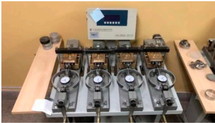
FIGURE 2 ZJ strain-controlled direct shear instrument.
