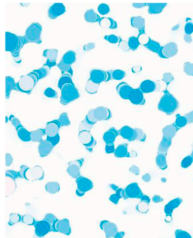
FIGURE 3 Schematic showing the pore radius location of the 2D image, pure white shown in solid pixels, and different depths of blue represent the process of locating the pore radius.
