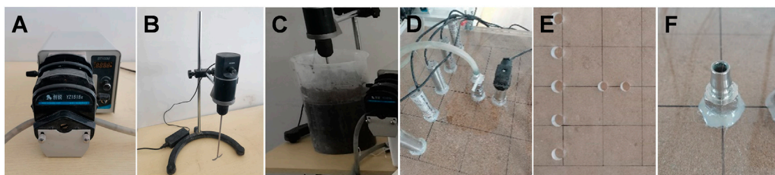
FIGURE 2 Grouting module. (A) Slurry pump, (B) slurry mixer, (C) slurry storage tank, (D) grouting pipe, (E) grouting hole, and (F) pipe hole connector.
