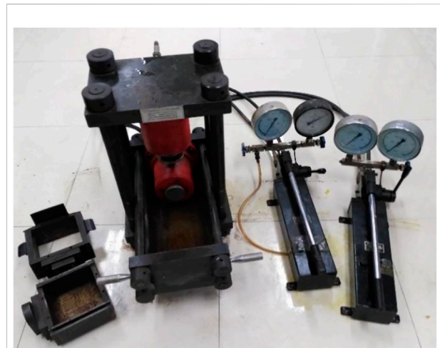
FIGURE 3 Direct shear test equipment picture.
