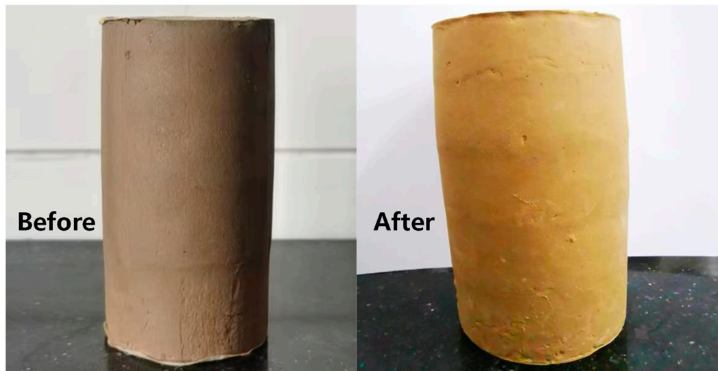
FIGURE 5 Soil bulging deformation of sample 3 after loading deviator stress q=300 kPa.
