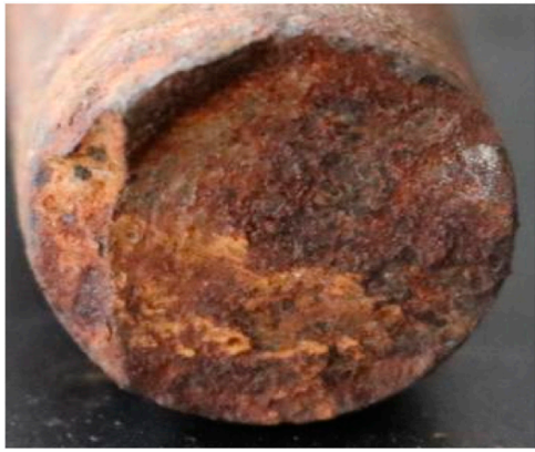
FIGURE 1 Fatigue cross-sectional shape of the pumping rod.
