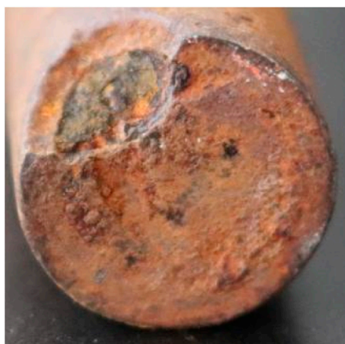
FIGURE 3 Fatigue cross-sectional shape of the pumping rod.
