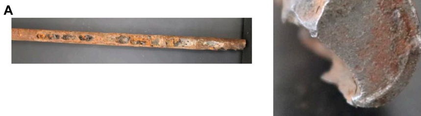
FIGURE 2 Fatigue cross-sectional shape of the pumping rod.
