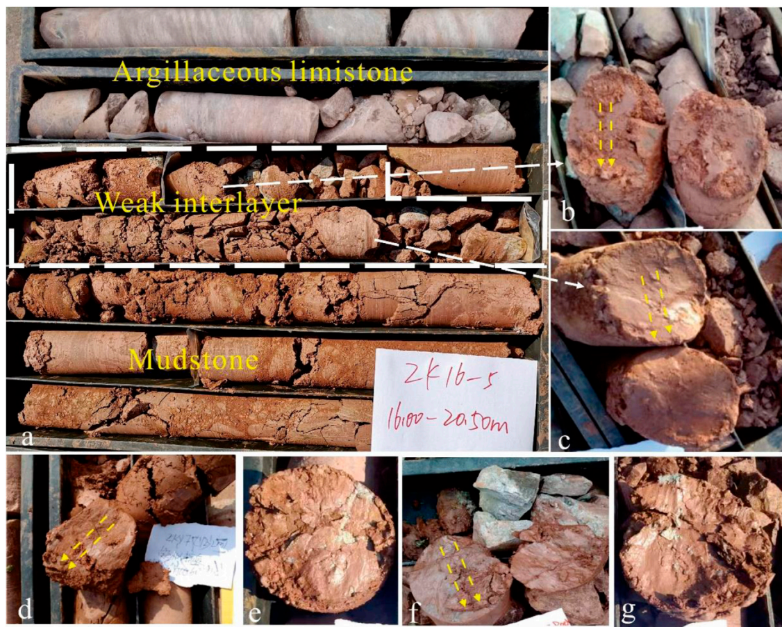
FIGURE 4 (A) is a weak interlayer in the sliding zone composed of broken mudstone and argillaceous limestone, which is revealed in Zk16, located at 17.5–18.6 m with a thickness of 1.1 m; (B,C) are argillaceous limestone and weathered mudstone, as revealed in Zk16, with respective depths of 17.7 m and 18.1 m; and (D–G) are revealed in Zk3, Zk7, Zk8 and Zk9, respectively, and contain many polished surfaces and slickensides.
