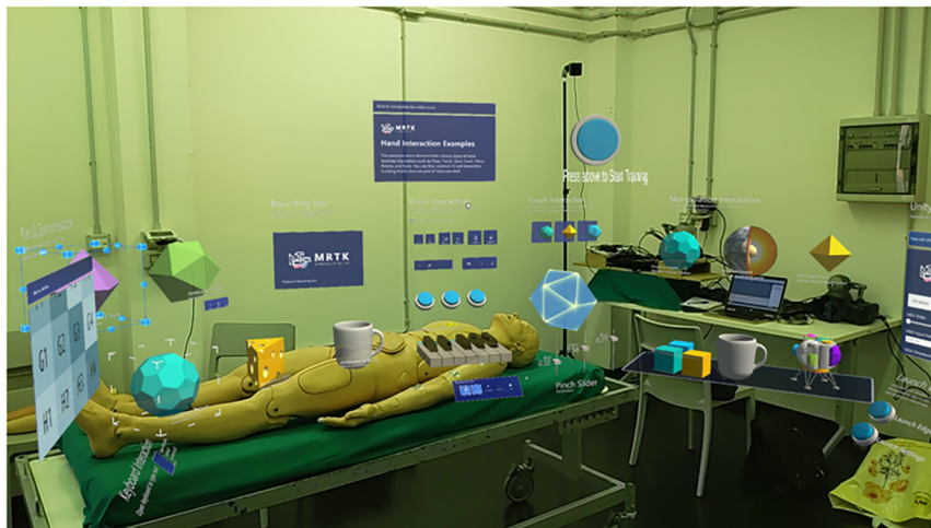
FIGURE 4 Demo session. It allows the user to get familiar with the application, and its interactions possibilities, such as grabbing and releasing virtual objects, QR codes, pressing virtual buttons.
