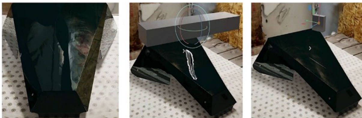
FIGURE 16 Left image shows the Sierra RX3 defect-free part (CAD), while right images Show Decals projecting synthetic scratches on the defect-free car part (Nvidia defect detection Omn (2022c) ).
