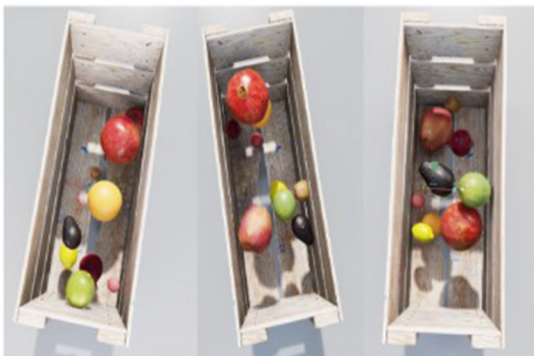
FIGURE 15 Domain randomization using Nvidia replicator generating three different scenes using the same assets [The Omniverse replicator Huynh-The et al. (2023)].
