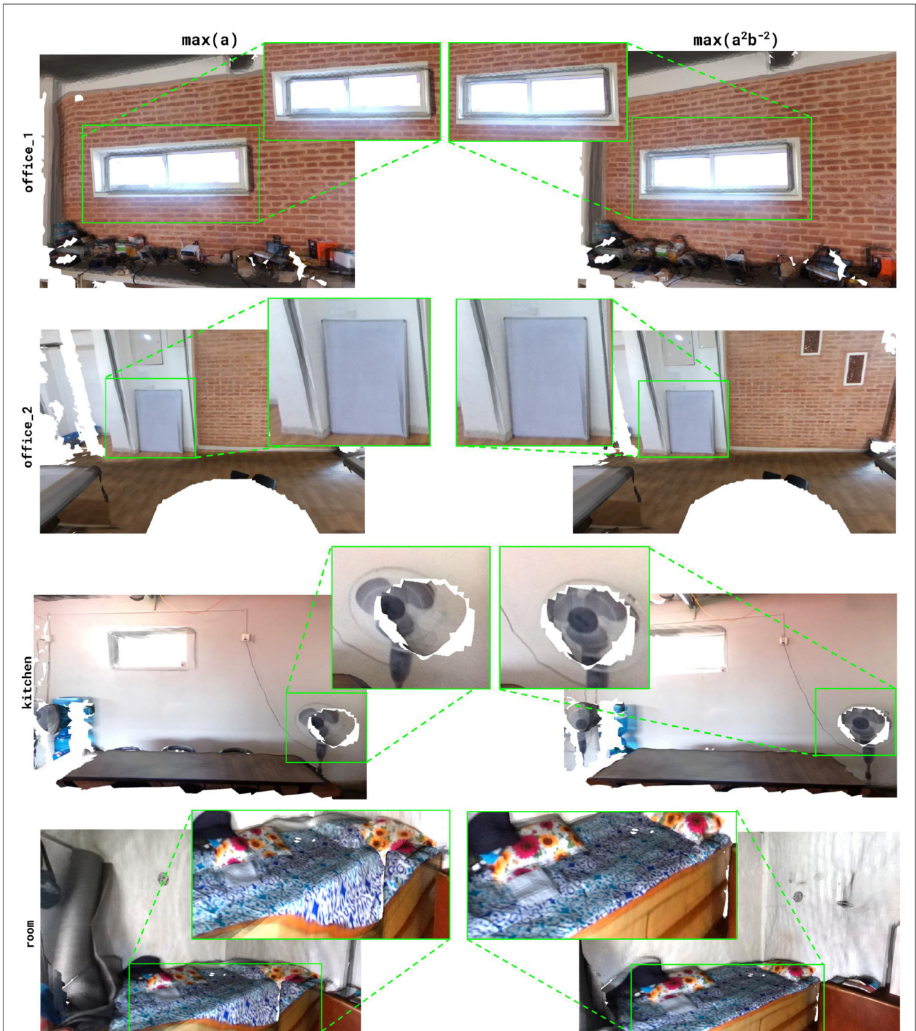
FIGURE 7 Comparison of texture alignment with 3D mesh using the transformations obtained with metrics \max(a) and \max(a^2b^{-2}) . The metric \max(a^2b^{-2}) yields more precise alignment than \max(a) . The missing triangle mesh regions (white) are due to the holes in the input 3D mesh which we later compensate for using the hole-filling algorithm as described in the Appendix 1 .
