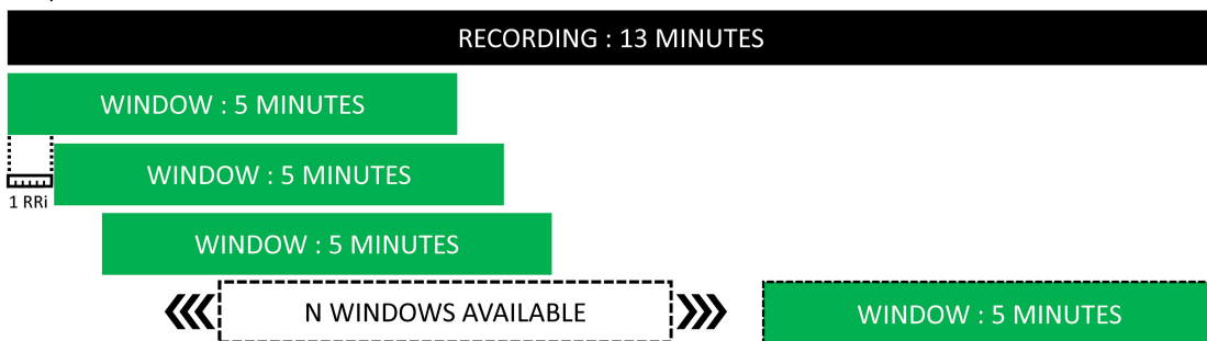
FIGURE 9 Baseline windowing optimization. (A) default windowing behavior for the baseline recording. (B) implemented baseline windowing algorithm. Moving reading frame every RRI logging every sequential window. Selects the highest quality 5-min window within a recording.
