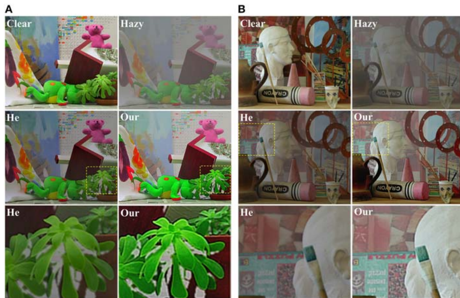
FIGURE 9 | Comparison with He's method on two synthetic hazy images. (A) Teddy image, (B) Art image. For each of (A,B), the top row shows the clear image and the image added with haze, the middle row lists the results by He's and our methods, and the bottom row lists the enlarged local patches. The Teddy and Art images are downloaded from http://vision.middlebury.edu/stereo/data/ .
