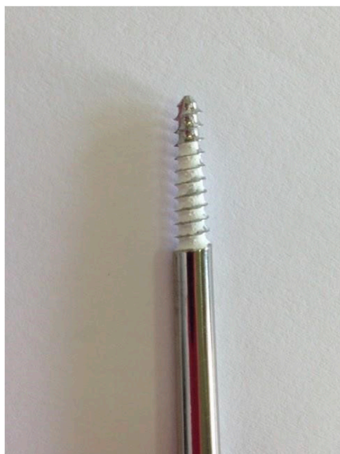
FIGURE 5 Image of the bone implant screw coated with the commercial HA deposited.
