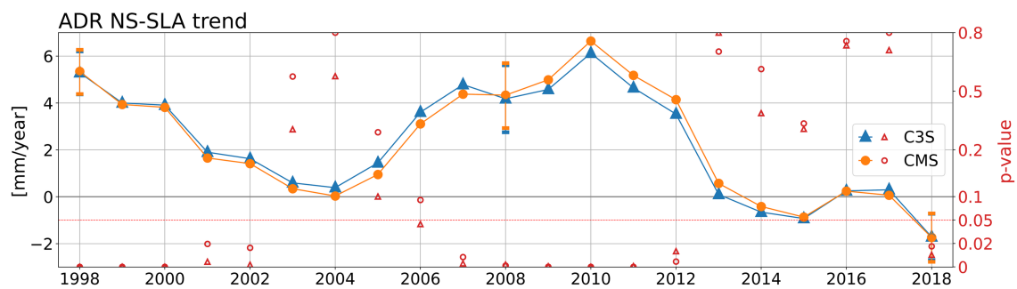
FIGURE 8 Timeseries of NS-SLA decadal trend values and correspondent statistical significance, computed over sliding windows shifted of 1 year over the period 1993–2022 in the Adriatic Sea. CMS and C3S values are represented by circles and triangles, respectively. Continuous lines show the evolution of trend values across each decadal window, while red markers indicate the correspondent statistical significance. The threshold p -value of 0.05 is shown as a dashed red line, corresponding to a confidence interval of 95%. Error bars represent the trend uncertainty, based on the bootstrap procedure, computed for the decades reported in Table 2 (1993–2002, 2003–2012, 2013–2022).
