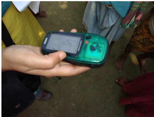
C Step 3: Geographical Positioning System (GPS) meter taking and saving the longitude and latitude location of each interview conducted in the two villages of the Bhola and Satkhira Districts for GIS analysis to create maps and locate the interviewer's position.
