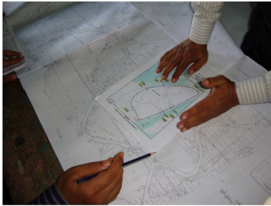
A Step 1: Char Kukri Mukri Union Map of Bhola District placed upon Mouza (villages) plot maps of that Union for matching the village's names and locations.
