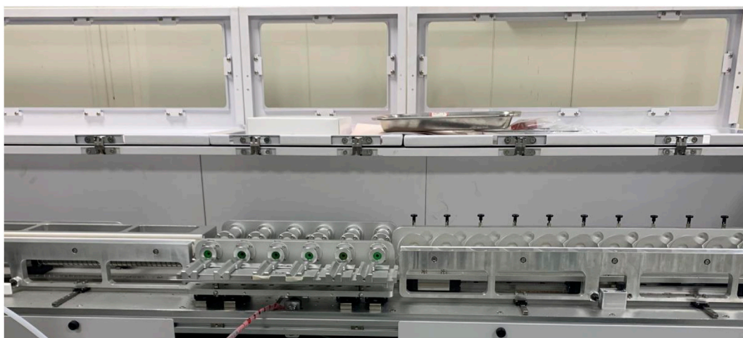
FIGURE 4 i-MAC600A array type multi-port puff-by-puff smoking machine.
