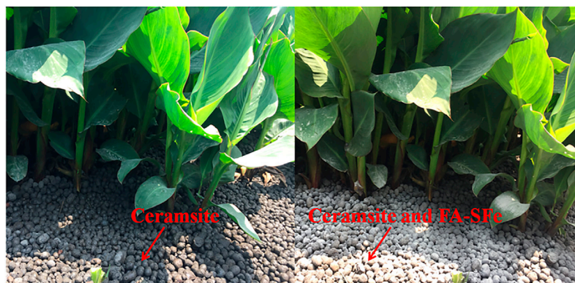
FIGURE 2 CW fillers with ceramsite and the mixture of ceramsite and FA-SFe.
