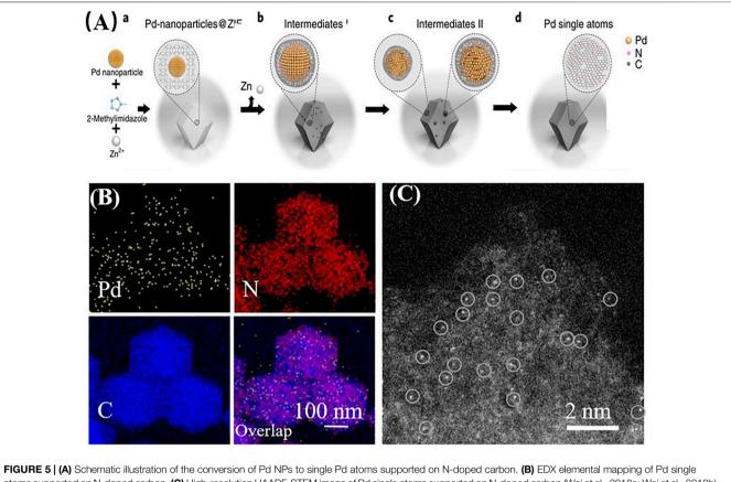
atoms supported on N-doped carbon. (C) High-resolution HAADF-STEM image of Pd single atoms supported on N-doped carbon (Wei et al., 2018a; Wei et al., 2018b). Reproduced with permission from (Wei et al., 2018a) Copyright 2018, Nature Publishing Group.
