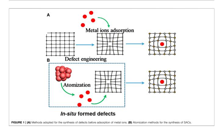
electronic configurations of the highly dispersed atoms can be tuned by modifying the coordination environments, resulting in a class of materials with unique properties (Huang et al., 2012; Deng et al., 2015; Fei et al., 2015; Xiao et al., 2019; Lei et al., 2020). The distinctive properties of the SACs have attracted considerable interest, especially in the area of catalysis.
