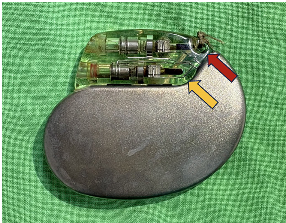
FIGURE 1 The dark brown discoloration of the RA (red arrow) and RV (yellow arrow) pin ports.
