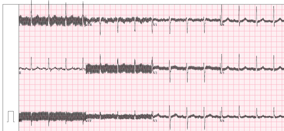
FIGURE 2 Sample ECG with electromagnetic interference-like artifact.
