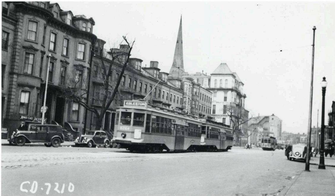
FIGURE 4 | 1930s Boston streetcar. A two-car train of center-entrance streetcars on Tremont Street at Upton Street (just north of Dartmouth Street), probably in the 1930s. From City of Boston Archives, West Roxbury, USA, via Wikimedia Commons ( https://www.commonswiki.org/wiki/File:Streetcars_on_Tremont_Street_opposite_Upton_Street,_1930s.jpg ).
