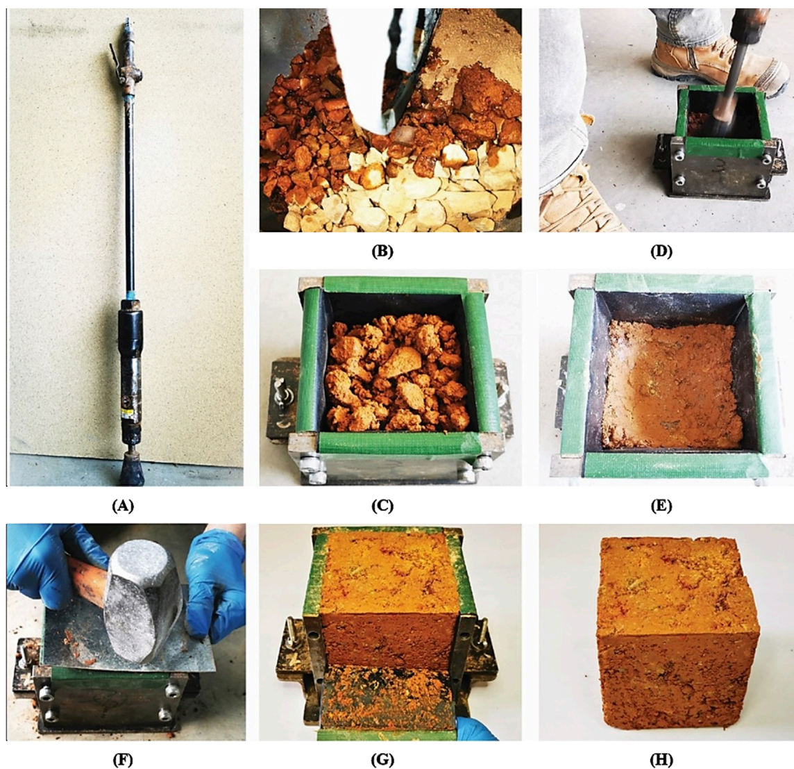
FIGURE 4 RE sample preparation process: (A) Kawasaki KPT-2L rammer; (B) soil mixing; (C) first layer of soil before ramming; (D) pneumatic ramming; (E) first layer of soil after ramming; (F) detailed compaction of the final top surface; (G) demolding the RE sample; (H) fresh sample after demolding.
