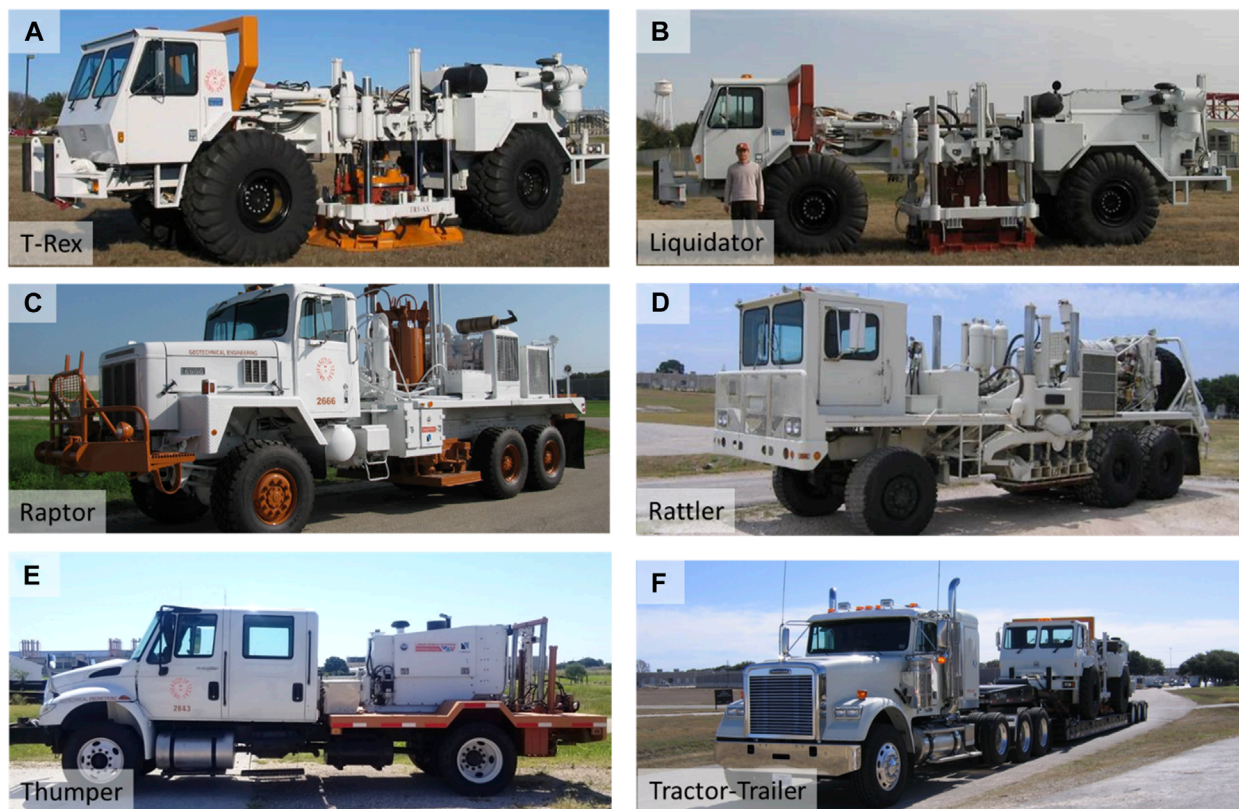
FIGURE 1 Photographs of the five mobile shakers and tractor-trailer rig available at NHERI@UTexas: (A) High-force, three-axis shaker called T-Rex, (B) Low-frequency, two-axis shaker called Liquidator, (C) Single-axis, vertical shaker called Raptor, (D) Single-axis, horizontal shaker called Rattler, (E) Urban, three-axis shaker called Thumper, and (F) Tractor-trailer rig, called the Big Rig, loaded with T-Rex (after Stokoe, et al., 2017 ).
