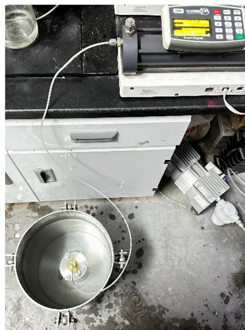
FIGURE 8 Assembly of the inner chamber under air-free water.
