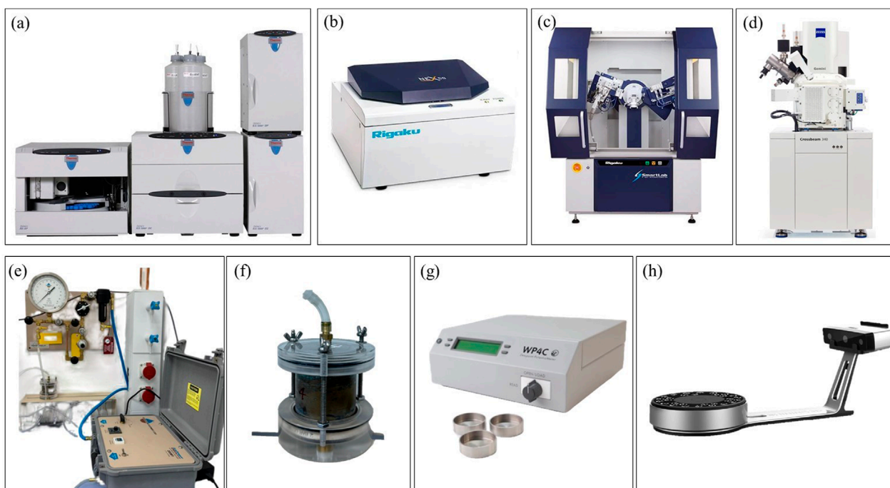
FIGURE 3 Experimental tests: (A) Dionex ICS; (B) Rigaku NEX CG-XRF; (C) Rigaku Smartlab-XRD; (D) SEM JEOL JSM IT200; (E) pressure controller system with automated air pump; (F) Tempe cell; (G) WP4C up to 300 MPa; (H) Einscan SP V2 3D scanner.
