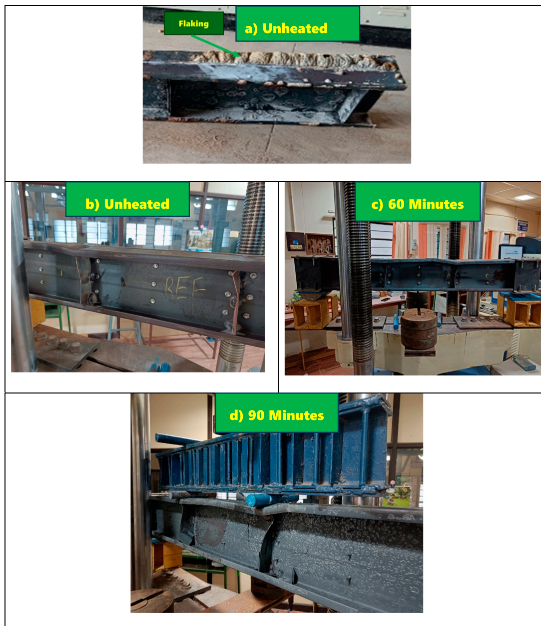
FIGURE 4 (A) Specimen after heating, (B–D). Failure pattern of specimens.
