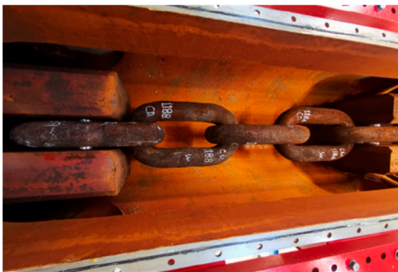
FIGURE 4 The general and pitting corrosion of mooring chains (Mendoza et al., 2022).
