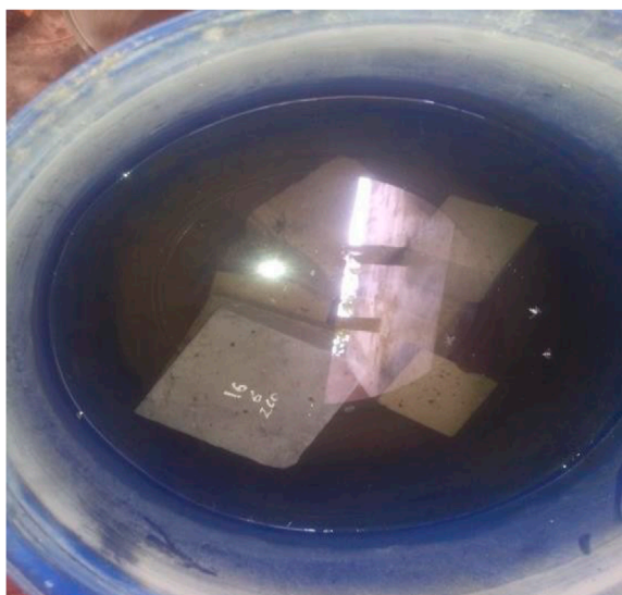
FIGURE 10 Specimens immersed for Water absorption test.
