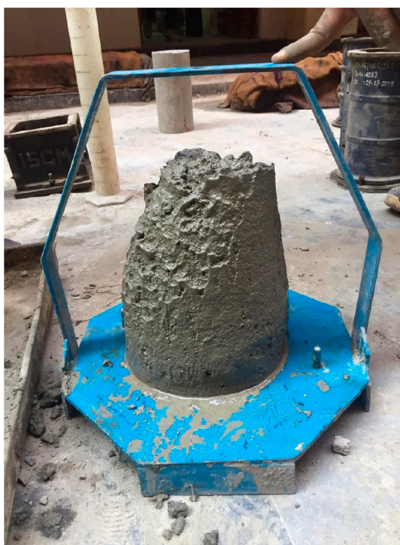
FIGURE 3 Slump cone test of GPA concrete.
