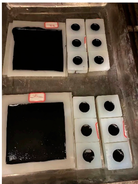
FIGURE 3 Asphalt residues obtained from the low-temperature evaporation method.
