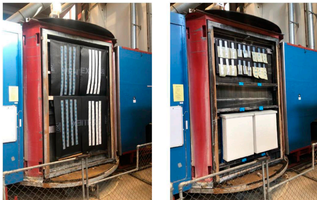
FIGURE 11 Test specimens in the climate carousel.
