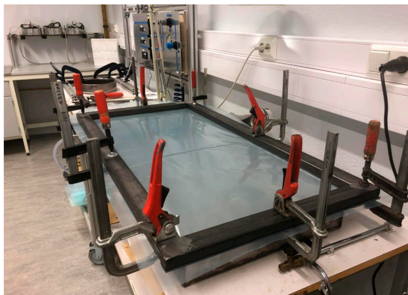
FIGURE 8 Test stand leakage evaluation setup using eight clamps.
