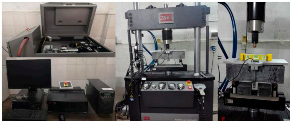
FIGURE 2 Mechanical test setup for measurement of UHPC specimen fatigue strength during cyclic flexural loading.
