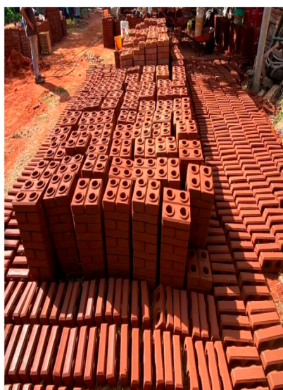
FIGURE 13 Compressed earth block sections—construction and material detail.
