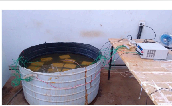
FIGURE 4 Accelerated corrosion process using power supply.
