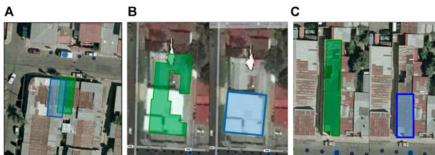
FIGURE 10 Difficulties with polygons highlighting building footprints. The color green denotes the polygon with error and the color blue denotes the corrected polygon. (A) corresponds to a position error, (B) to a geometry error, and (C) to a size error.
