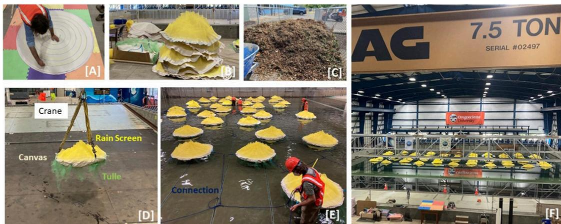
**FIGURE 4** | Construction of the individual mats and the network, from (A) cutting and marking canvas to 5 ft diameter, (B) sewing rain screen (yellow) to the top canvas piece and tulle (light green) with a webbing triangle (light blue) to the bottom piece, (C) using wood discard fragments to stuff the units, (D) lifting a stuffed and sewn unit into the basin where (E) it is tied to other units using nylon rope (dark blue) to finally set the (F) completed network in 1.37 m of water depth.
