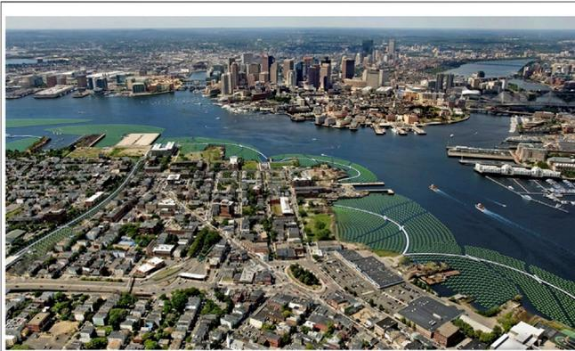
**FIGURE 1** | Aerial view of a rendering of the Emerald Tutu (green circles) surrounding East Boston, MA. The white strips represent walkways through the mat which can be used by community members during calm weather.
