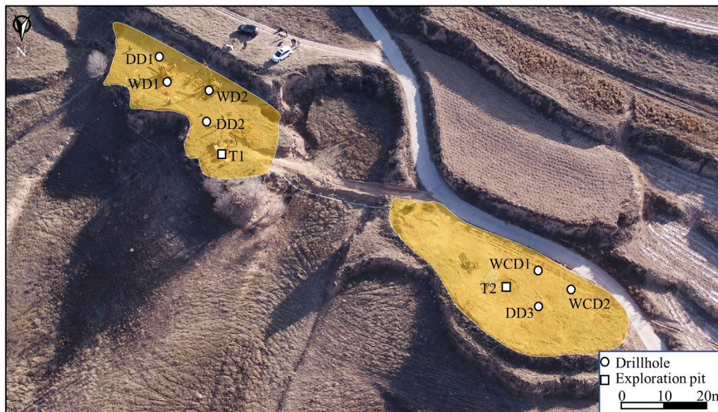
FIGURE 1 | Site investigation with seven drillholes (DD1, DD2, DD3, WD1, WD2, WCD1, and WCD2) for SPT tests and two exploration pits (T1 and T2) for collection of undisturbed samples.
