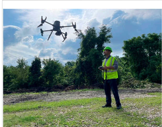
FIGURE 2 Collecting data using DJI Matrice 300 RTK drone.
