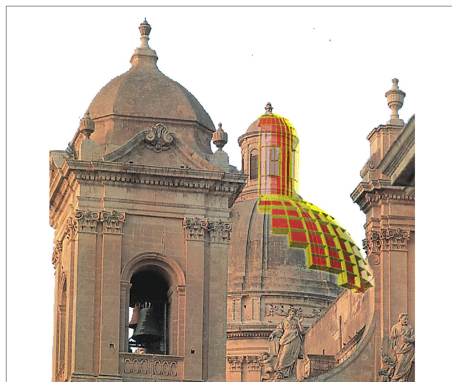
FIGURE 1 | A simplified qualitative representation of the use of shell macroelements for curved geometry monumental structures modeling (Calió et al., 2010).
