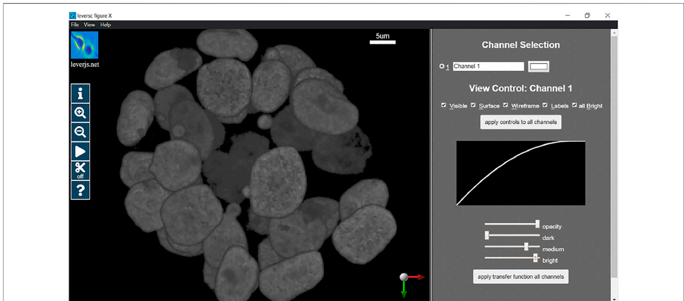
FIGURE 2 | LEVERSC render parameter selection interface. Colors, alpha blending and intensity mapping transfer functions are all fully controllable via the user interface and the API.
