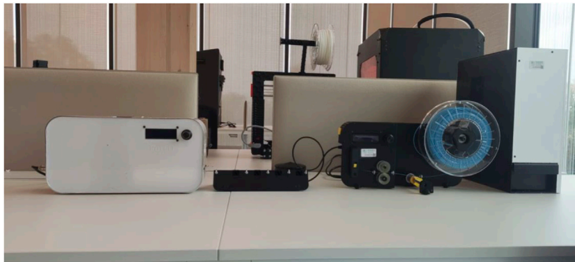
FIGURE 4 Extrusion and spooling process. From left to right: extruder, cooling system and spooler.
