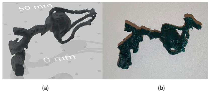
FIGURE 13 (A) 3D model of aneurysm (B) 3D printed aneurysm.
