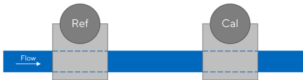
FIGURE 3 Schematic representation of the master meter method for flow sensors.
