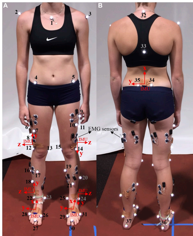
FIGURE 1 Pictures of the front (A) and back (B) of a participant, illustrating markers' placement (numbered in the image) and sensor locations (IMU axes depicted in red). The study did not utilize data from the Electromyography (EMG) sensors.
