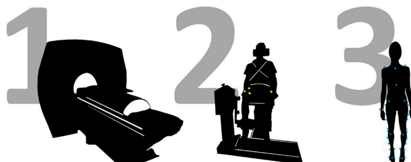
FIGURE 1 Schematic representation of the study protocol, involving three different data acquisition sessions. First, full lower limb MRI data are acquired on a 3T scanner. Then, a MVIC test is performed on a dynamometer, in various knee configurations (i.e., with knee flexed at 75° and 90° degrees), whilst recording surface EMG data from eight major lower limb muscles. This includes the delivery of a superimposed neuromuscular electrical stimulation. Last, a gait assessment is conducted.
