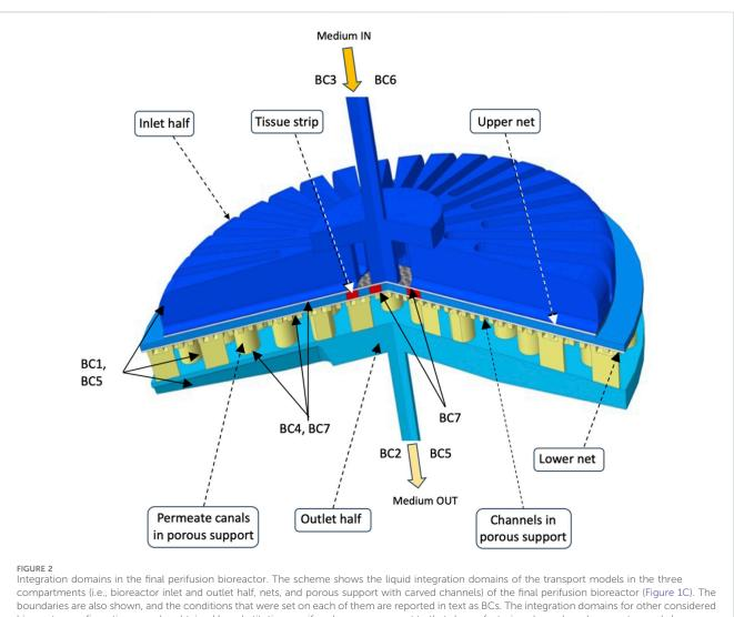
bioreactor configurations may be obtained by substituting a uniformly porous support to that shown featuring channels and permeate canals (e.g., Figure 1B), and by additionally removing the lower net below the tissue strips (e.g., Figure 1A). Details can be found in Section 2.
