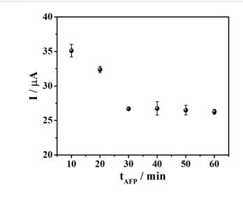
A plot between AFP incubation time and DPV current responses of TB after binding with 50 ng mL<sup>-1</sup> AFP in PB (0.010 M, pH 7.0).
