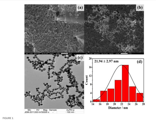
SEM images of (A) naked and (B) PEI-AuNPs modified SPCEs (C) TEM image of the synthesized PEI-AuNPs and (D) corresponding histogram of size distribution profile (21.94  $\pm$  2.97 nm).
