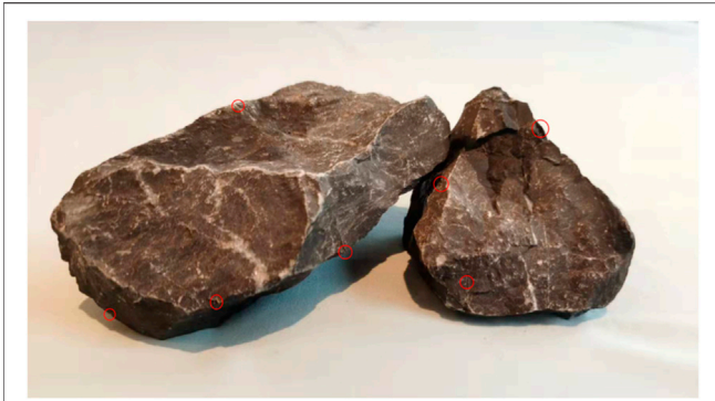
FIGURE 4 | There are many small indentations on the surface of the aquarium stones (small red circles). In their MRI image, those indentations that meet the CAF standard are used as characteristic areas, to improve the measurement accuracy.
