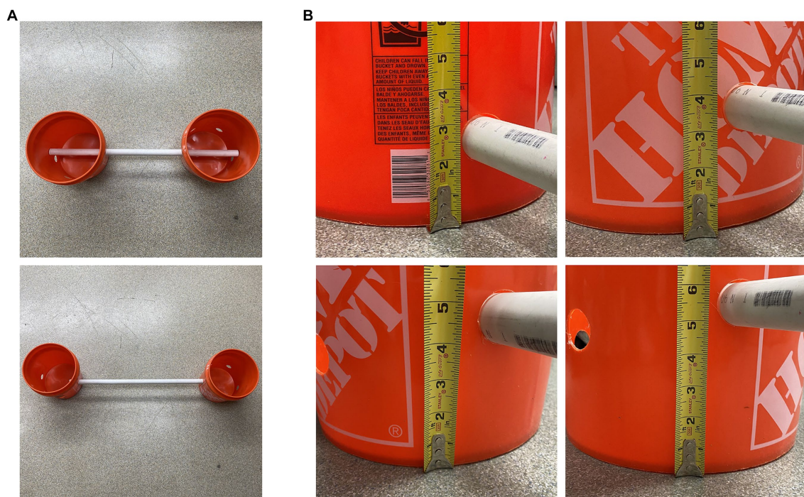
FIGURE 2 Example images showing the adjustable length and height of the ladder rungs. (A) The upper picture shows the shortest length of the rung, and the lower picture shows the longest length of the rung. (B) From the top left to the bottom right, the rung heights were at 3 in, 4 in, 5 in, and 6 inches with holes drilled with spaces around each bucket.
