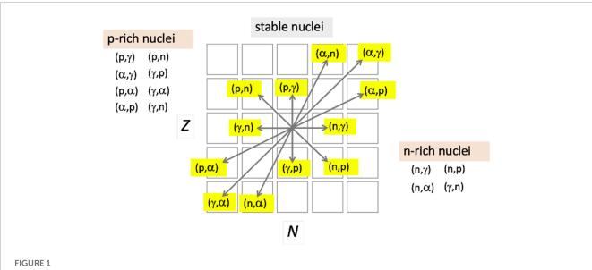
Reactions of importance for nuclear astrophysics shown on the N-Z plane for stable nuclei (center), and as lists for proton-rich nuclei (right), and neutron-rich nuclei (left).
