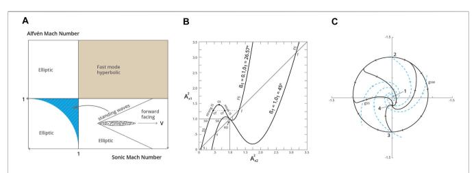
**FIGURE 1** Standing waves and shocks in MHD: (A) Standing upstream-facing slow mode waves in blue shaded region; (B) Slow, intermediate, and fast shock wave jump properties from upstream (1) to downstream (2) conditions; angle  $\theta_1$ , is between shock normal and upstream magnetic field (C) Example of predicted magnetic hodogram for a shock structure.
